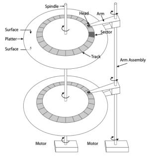
As seen in the picture above, magnetic disks have lots of moving parts, which can lead to many physical issues. Compared to flash memory in the next section, the read/write times are a lot slower. However, they are much cheaper compared to flash memory, offering a better data size to price ratio.
